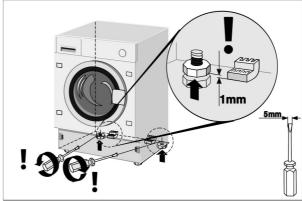
Once the appliance is in position in the kitchen, the height of the rear feet has to be increased so that the appliance no longer stands on the skids. After adjusting the rear feet, level the appliance and fix the front feet at the height required.
